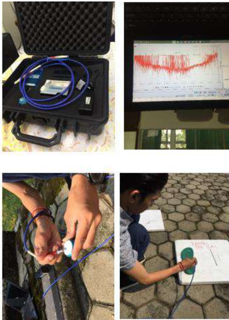
Figure 4. Spectral measurement of plastic debris using Ocean Optics USB 4000
